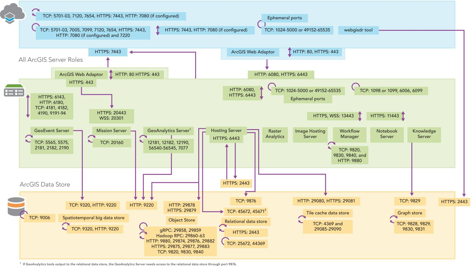
Ports need to be available on individual machines. No external communication is needed. Ports used for communication between machines in the same site or data store. For example, all machines in a single ArcGIS Server site or a single object store.
